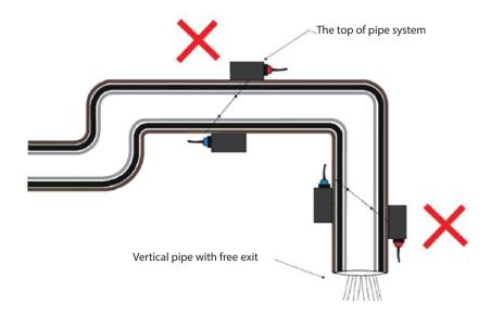
• For the open pipe or half full pipe, the transducers should be installed at the bottom of U pipe.
