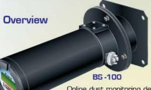
Online dust monitoring device using the mainstream technology of laser back-scattered light principle with imported core components. BS-100 is mainly used for continous monitoring of various sources emissions of particulate matter concentrations. It can be either equipped with CEMS, or connected with dust monitoring network by a shared set of data acquisition and processing background.
