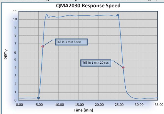
responsive sensor, coupled with a volume-optimized internal sampling system means that the QMA2030 will give a 63% response to a step change in moisture in less than 2 minutes, more than twice the speed of comparable QCM analyzers. 95% response is achieved in less than 5 minutes, as the graph below left demonstrates.
