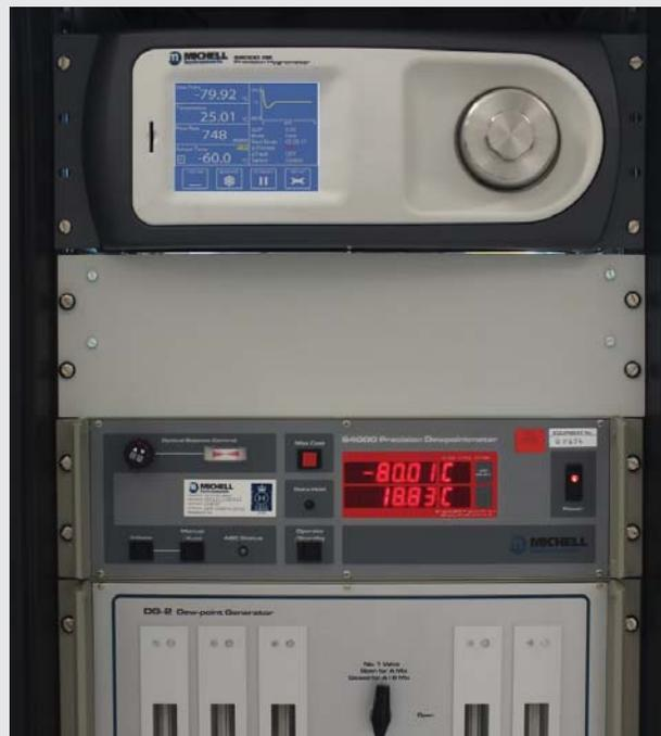
The S8000 RS provides a reliable reference for dew-point calibrations
