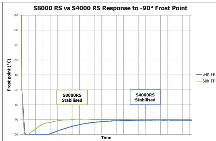
The graph opposite compares response speed of the S8000 RS with its predecessor, the S4000 RS, to a sample of -90°C frost point (-130°F frost point).
