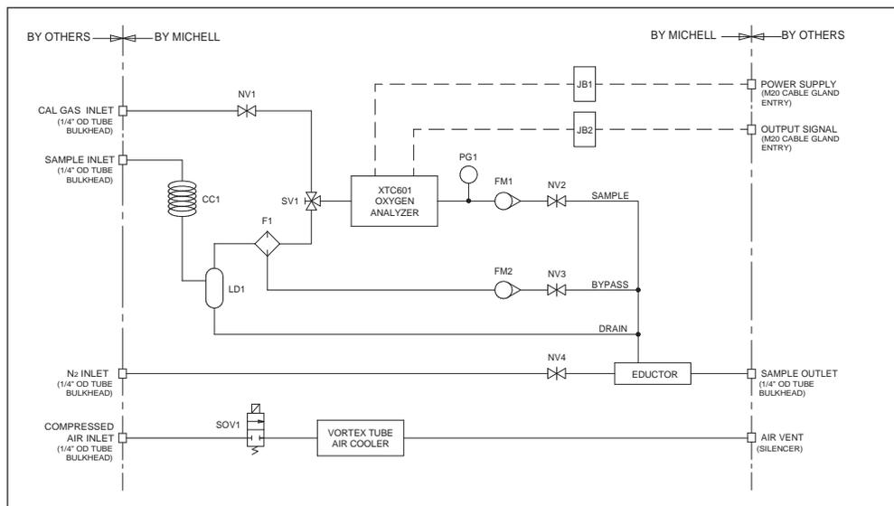
The sampling system shown is for use with "misty" gases sampled in a hazardous area. It is one of the more complex sampling systems available.
